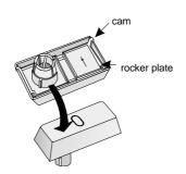
Insert the key cap in the keyboard and press firmly into place.
